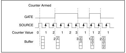
Figure 7-10. Buffered Semi-Period Measurement
